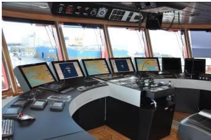
The Synapsis INS will be delivered in accordance with IMO's INS Performance and Test Standards as specified in MSC.252(83) and IEC 61924-2. Further, the 88 meter long vessel meets the demanding class notation DNV NAUT-OSV. These classification rules list specific requirements regarding bridge layout, redundancy and function with a focus on safe operation.
